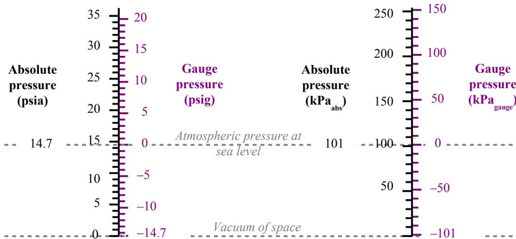
In U.S. Customary units, add 14.7 psi to convert from gauge to absolute pressure; in SI units add 101 kPa to convert from gauge to absolute pressure.
