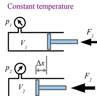
For example, let  $V_1 = 800 \text{ in.}^3$ ,  $p_1 = 25 \text{ psig}$ ,  $d = 10 \text{ in.}$ , and  $\Delta F = 100 \text{ lb.}$  Since the initial pressure is given in gauge pressure, we have to convert it to absolute pressure by adding 14.7 psi.
