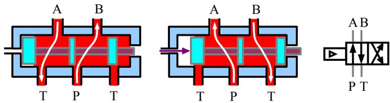
This valve needs some method to move it back to the left...it could be another pilot control, or it could be a cam, or a spring, or some other method.
