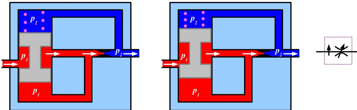
There are other types of valves that can compensate for pressure and temperature changes. This valve compensates for pressure. The fluid is flowing from left to right, past a spool, and through an adjustable throttle. The pressure upstream from
