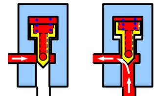
use a hollow poppet, so the excess goes back into the main flow.
