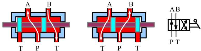
The symbol represents the flow paths inside the valve. In a hydraulic valve, the two tank ports are connected internally to a single fitting, so you only have one connection to make to your hydraulic line to tank.
