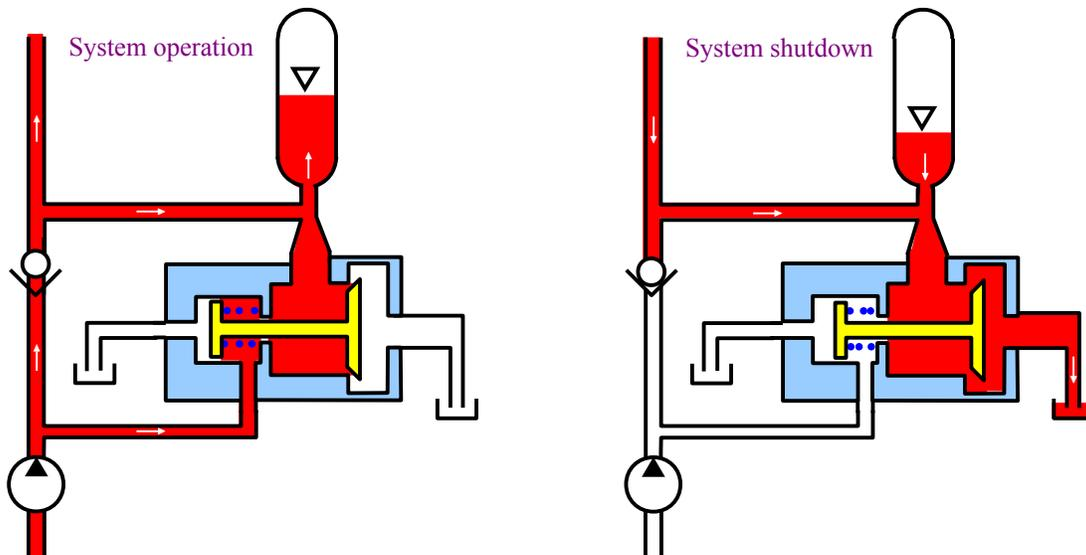
A hydraulic pump sends flow to the system, to the accumulator, and to the pilot line of the pilot-to-close check valve. When the pump is running, the accumulator builds up gas pressure. The pilot-to-close check valve is in the closed position. When the pump shuts down, we lose pressure to the pilot, so the pressure from the accumulator opens the valve to drain the accumulator and the rest of the system to tank. Notice the level in the accumulator is going down, and the gas expands.
