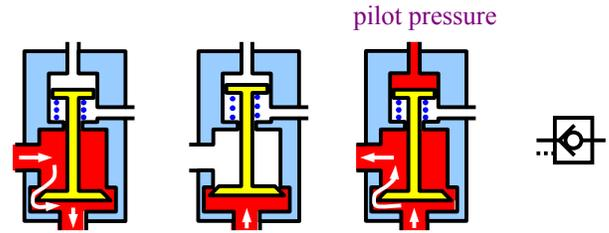
You could use this type of valve to hold a hydraulic cylinder locked in place until a main directional control valve is shifted.
