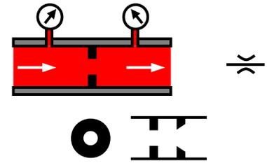
If we install a pressure gauge on either side of the plate, we'll find that the pressure drops as the fluid flows through the plate.
