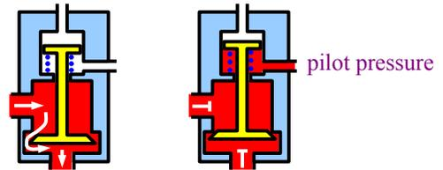
What we have is a valve which operates automatically to keep flow moving only in one direction, or it can be opened by remote control to allow flow in both directions, or it can be closed by remote control to prevent flow in any direction. This is a pretty useful flow control device.
