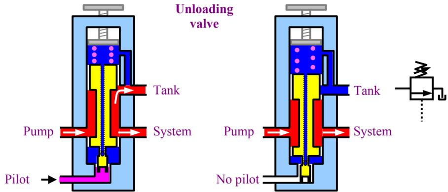
When the pilot pressure drops below a certain value, the spool is pushed down by the spring, and flow to the tank stops. All the flow goes to the system. The spool is hollow, so we can relieve the pressure above and below the spool as it moves up and down. The spring is adjustable, so we can set the required pilot pressure.
