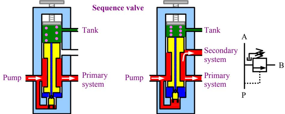
This symbol is a little different from the one in the book. The textbook symbol doesn't show both circuits, A and B. The increased pressure in the pilot line pushes the spool up, and opens flow to a secondary circuit, marked "B" on the hydraulic symbol. In the lab, circuit B is the second cylinder.
