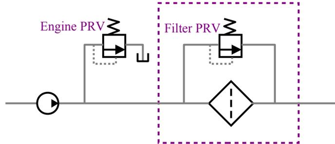
If you lose lubrication, you also lose bearings. The PRV in the filter is either a leaf spring or a coil spring that pushes a disk of paper or rubber against a hole.
