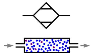
We remove moisture using a desiccant: a material that readily absorbs water from the air, like silica gel. The symbol for an air dryer has two lines parallel to the flow direction.
