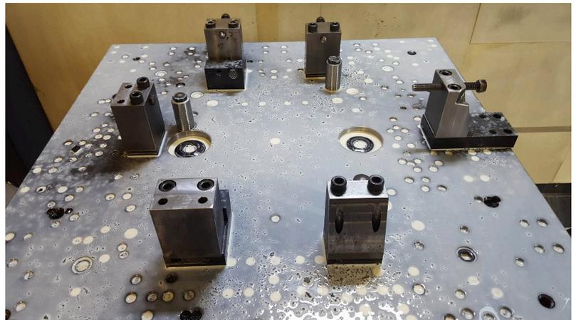
**Figure 1: A photo of the current op10 fixture. Note the many bolt holes and static blocks that add to the set-up time.**
