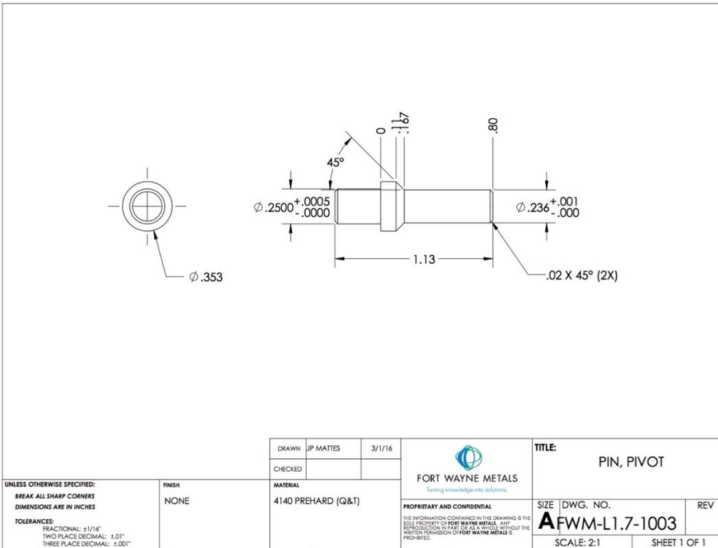
Figure 8 new pivot pin
