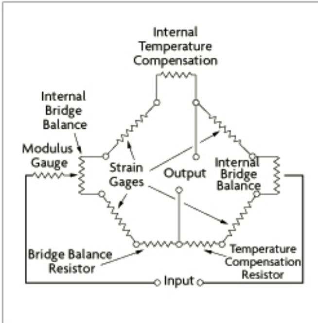
Figure 10 load cell internal circuit
