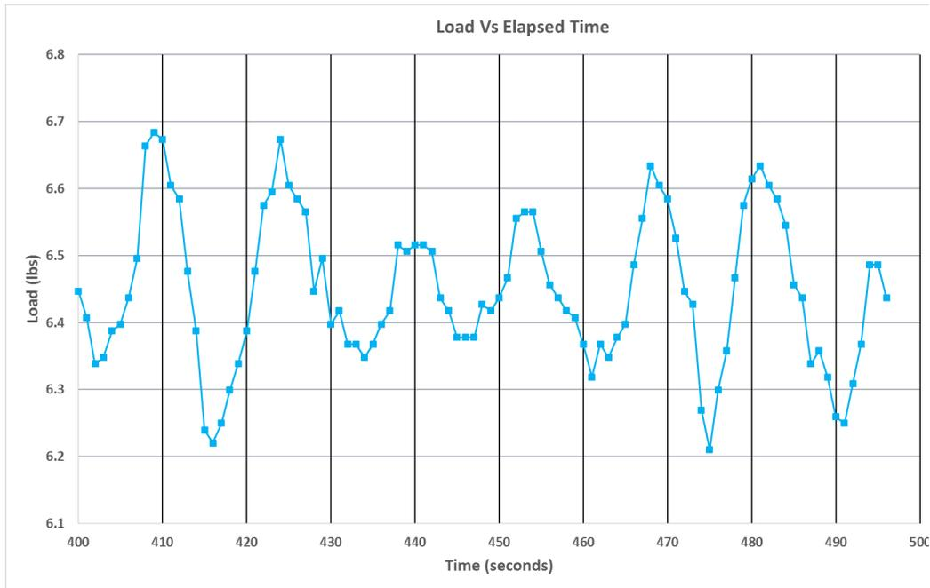
The second chart shows the data collected just after a die mark was observed in the wire. The data does look slightly different than the first chart, but no glaring variations appear.
