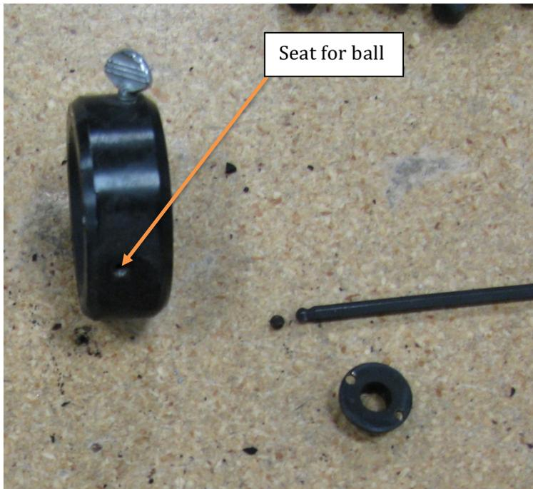
The ball is then compressed to support that side, by tightening a setscrew. This contains the ball axially and is adjusted to remove end play. It is then locked by a second setscrew that is perpendicular to the first. A clamp device locates on the shaft and allows initial adjustment. The knurled screw is then tightened to allow fine micrometer adjustment.
