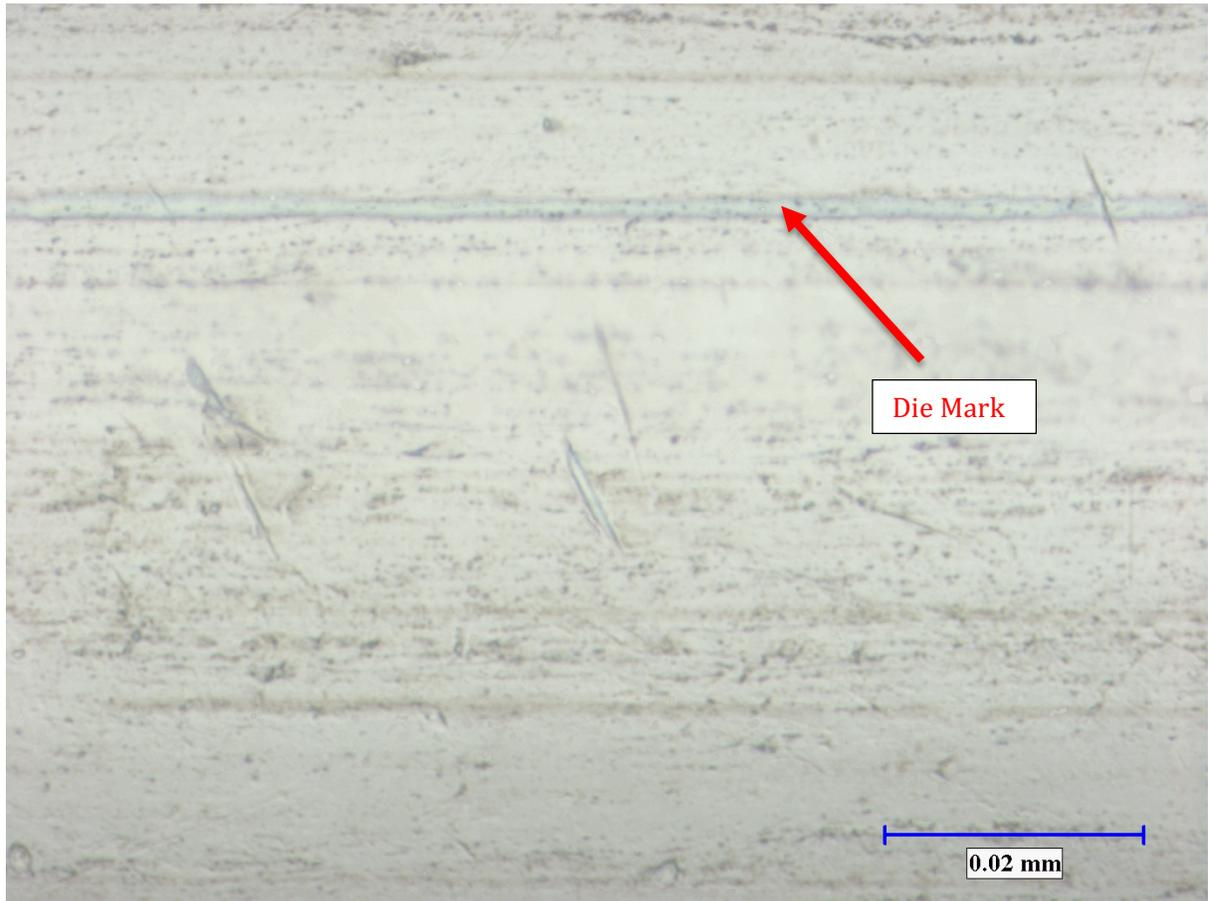
*Figure 12 magnified view of .0079" diameter wire with die mark defect*
