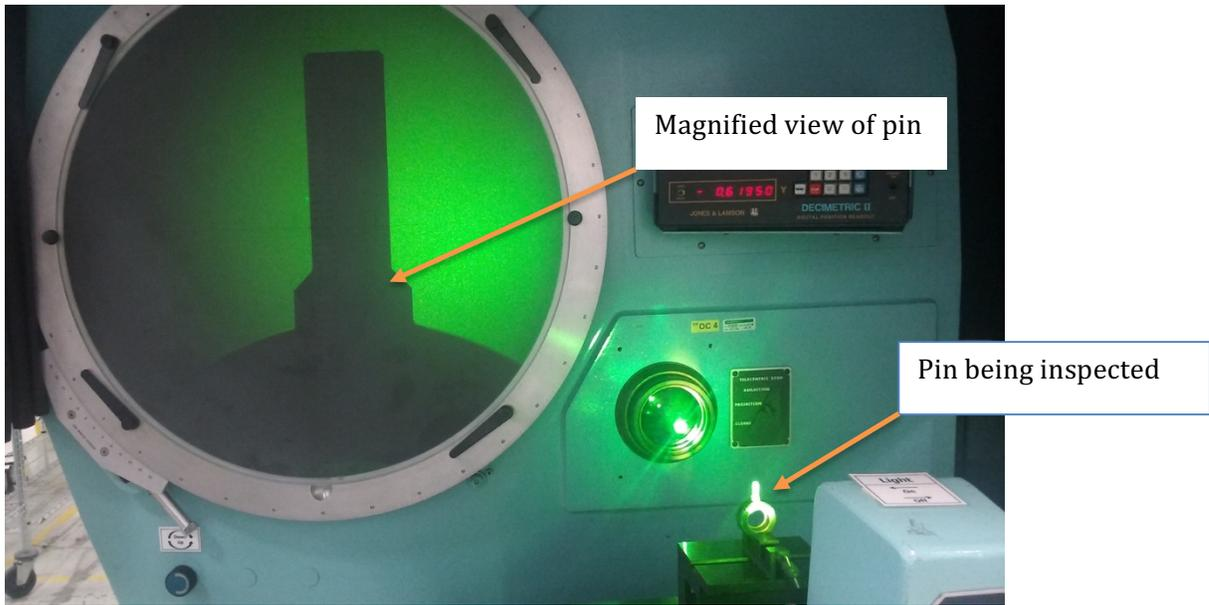
The existing pin is shown during the measuring process in Figure 7 (above).
