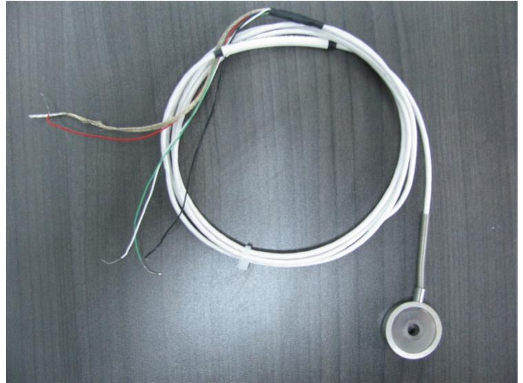
Figure 4 the load cell
