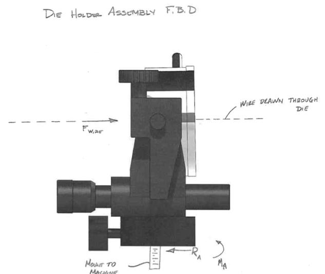
Figure 3 free body diagram
