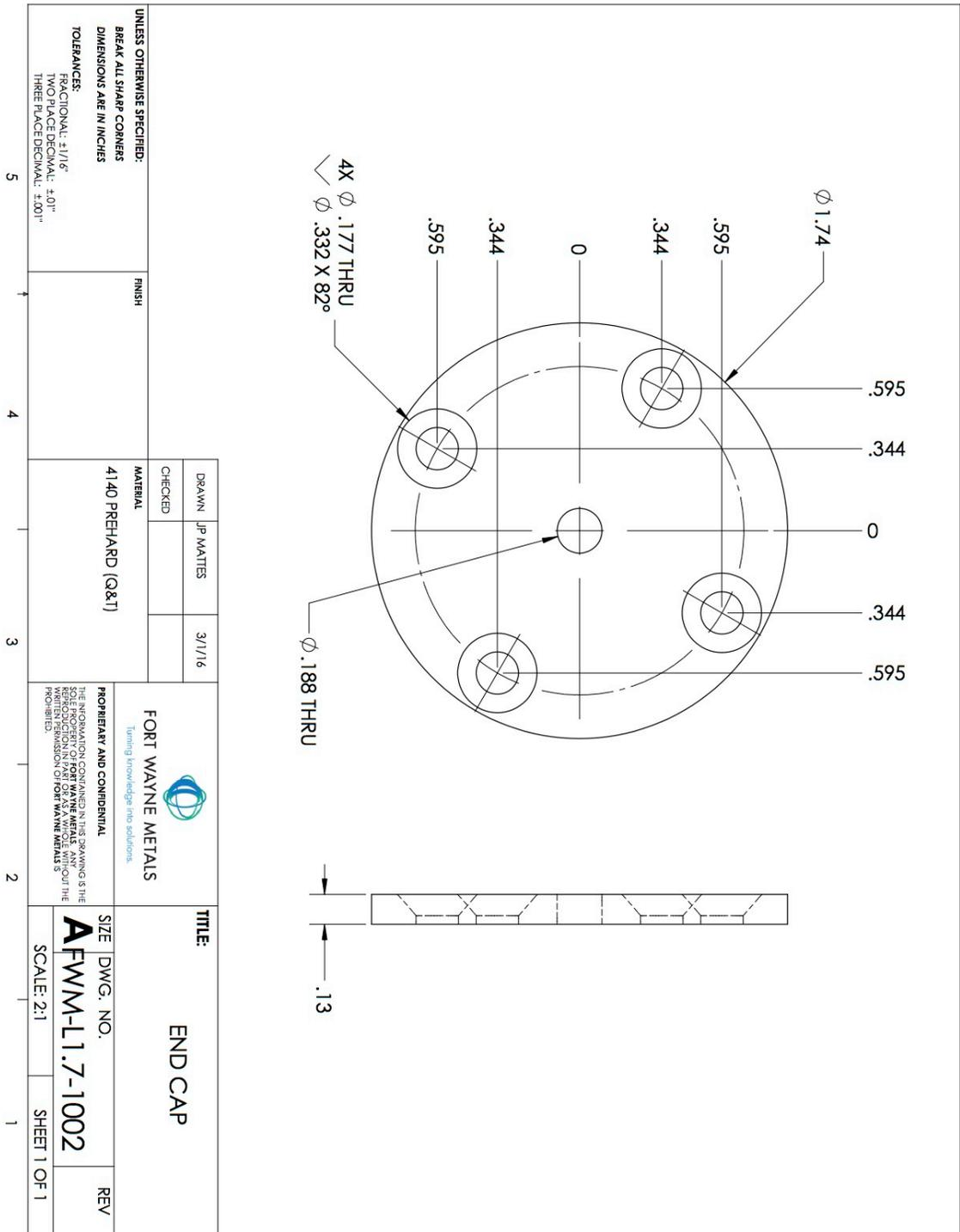
End cap, allows for load cell removal
