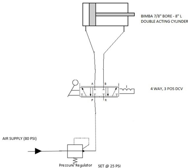
We also had to calculate how much the pan will weigh with it being full of chips and oil. The cylinder can lift approximately 15 pounds at 25 psi. We calculated we only need to lift 12.8 pounds based on the weight of a pan plus full load of oil and chips. Based on our calculations below the cylinder at 25 psi I should provide adequate pressure to raise and lower a full load of chips.
