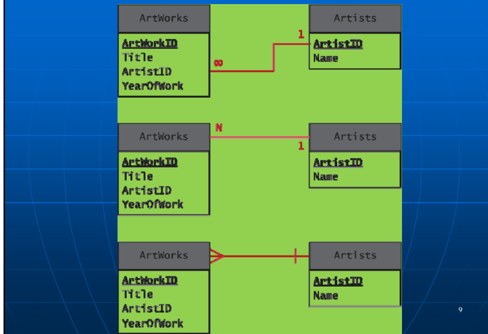
Figure 11.6 Diagramming a one-to-many relationship
