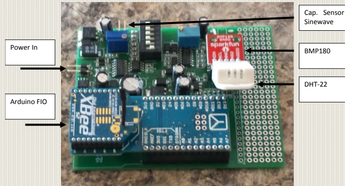
Wireless Sensor Node (Arduino FIO, XBee Transceiver & ASP)
