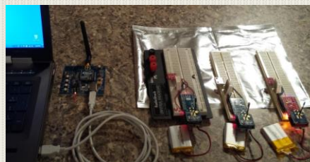
Network Coordinator + 3 Prototype Sensor Nodes
