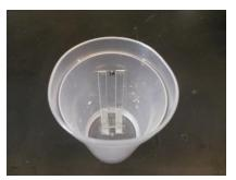
SnCl<sub>4</sub> sol-gel coated on glass plates with aluminum tapes. The sensor is soaked in NaCl solution for testing.
