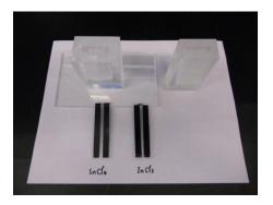
SnCl<sub>4</sub> and InCl<sub>3</sub> sol-gel coated on glass plates with carbon tapes. The carbon tape is black.
