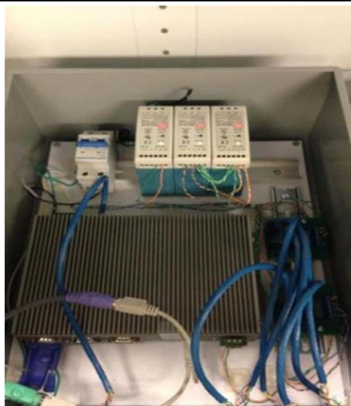
Embedded Computer Server Box with RS 485 Communication
