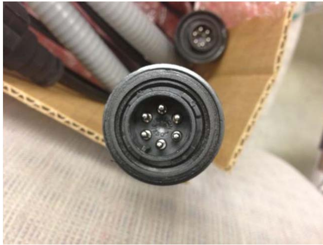
Figure 11: 6 pin Sensor Box Connection Wire for Power Supply and RS485 Communication Lines
