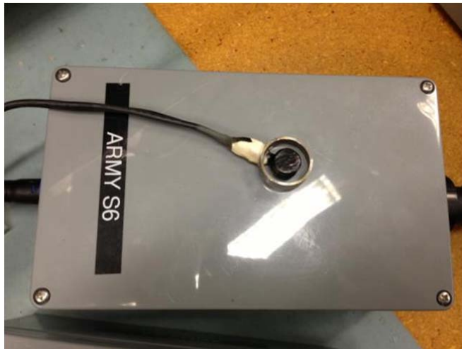
Figure 9: Tar-Coated Cylindrical Sensor6 and Sensor Box S6
