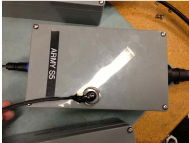
Figure 8: Coal-tar epoxy coated Cylindrical Sensor5 and Sensor Box S5
