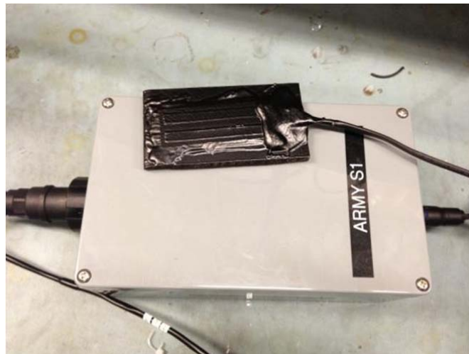
Figure 4: Coal-tar epoxy coated Sol-Gel Sensor1 and Sensor Box Army S1
