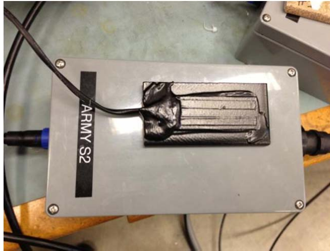
Figure 5: Coal-ta epoxy coated Sol-Gel Sensor2 and Sensor Box S2
