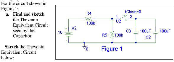
Write the values for the Thevenin equivalent resistance and voltage below:
