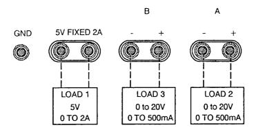
Connections for BOTH positive and negative supplies are shown below. Once again, the "A" and "B" supplies are variable and the "Fixed" supply is a constant 5V. All of these supplies can be either positive or negative supplies.
