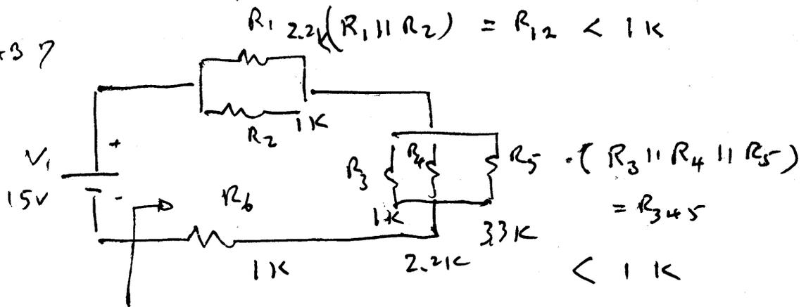
$R_1 \parallel R_2 = R_{12} < 1k$
