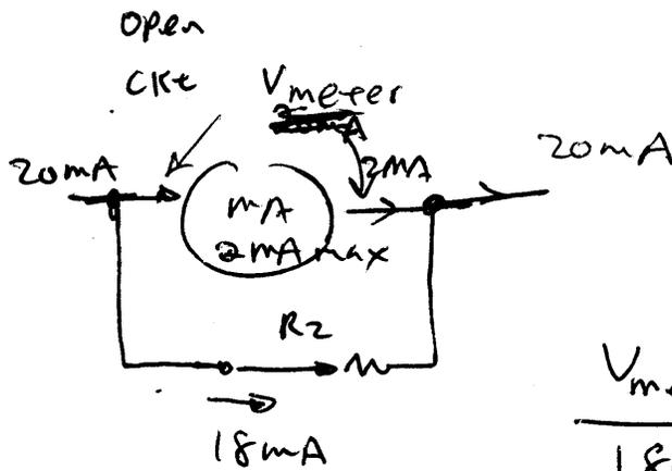
$$\frac{V_{meter}}{18mA} = R_2 \quad \text{design}$$
