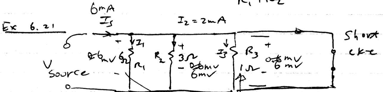
Step 1) Find  $V_{R_2} = I_2 \cdot R_2 = 2mA \cdot 3\Omega = 6mV$
