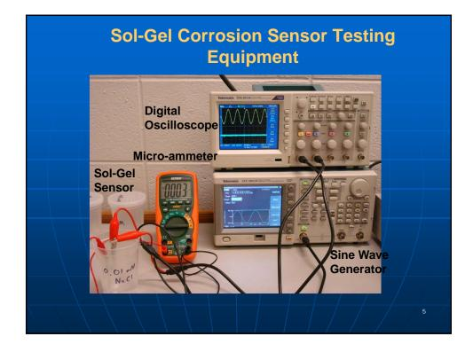
Sol-Gel Corrosion Sensor Testing Equipment Demonstration
