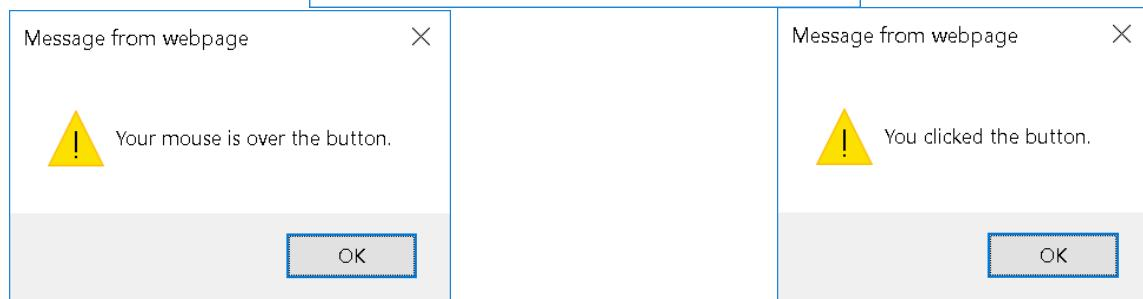
**Example 6-6:** An example shows how to call functions through the button controls and events.
